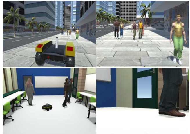
Figure 1: SEAN's rendering a world (left) and view of the scene from the robot's perspective (right). The outdoor city scene (top) and the lab scene (bottom) include dynamic pedestrians for studying social robot navigation.
