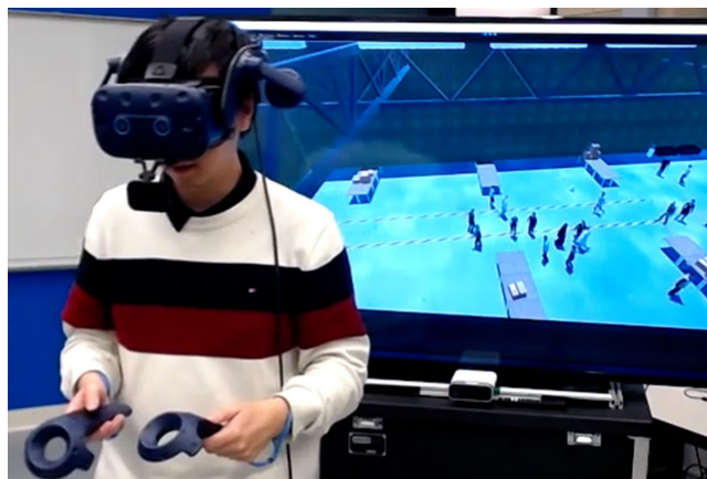
Figure 1: Our Virtual Reality (VR) demonstration system. A user controls an avatar through VR in the Social Environment for Autonomous Navigation (SEAN). A robot in the simulation guides them to a destination in the virtual world.
